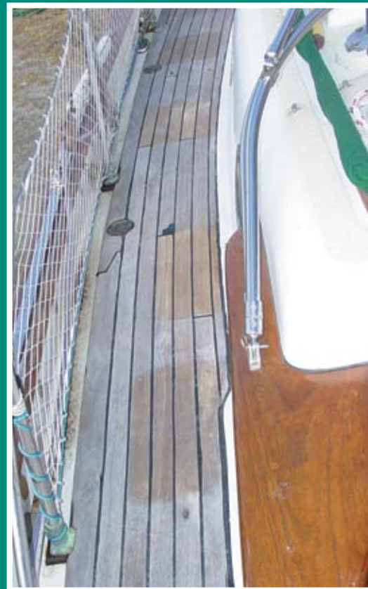
We sectioned off the deck of a Union 36, turning it into a teak checkerboard. The after-most test patch was cleaned with Star brite Teak Cleaner, followed by an area cleaned with Interlux Premium Teak Restorer.
